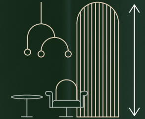
2.7-3m finished floor to ceiling height
